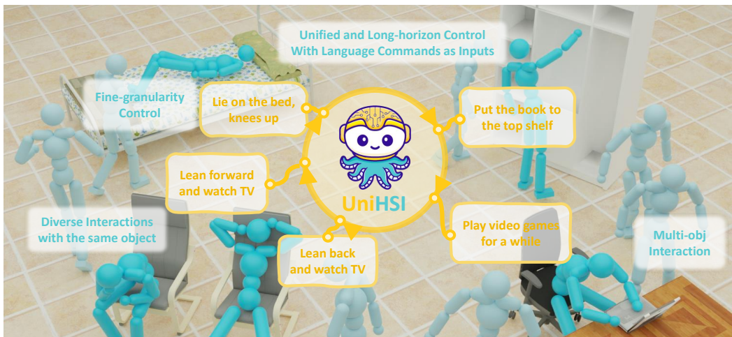
Figure 1: UniHSI facilitates unified and long-horizon control in response to natural language commands, offering notable features such as diverse interactions with a singular object, multi-object interactions, and fine-granularity control.
